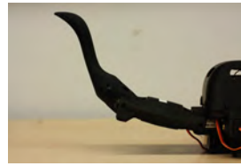
(c) The femur's position is raised twelve degrees from the position of contact.
