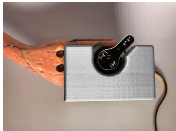
Figure 6: The 3D printed mechanical jig (grey) is placed on the motor and guides the coupling of the servo horn (black) to the proper orientation.
