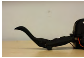
(b) The femur is lowered until it touches the flat surface at its lowest point. The PWM period of this point is recorded.
