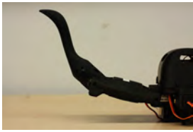
(a) The sequence for each leg starts with the Spyndra on a flat surface. The femur and tibia are raised to their maximum angles.
