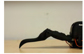
(d) Now, the tibia is lowered until it touches the flat surface at its lowest point. The PWM period of this point is recorded.
