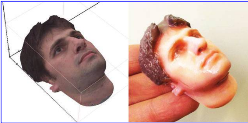
Figure 1. A full color texture AMF file in viewer ( left ) printed directly on a CONNEX3 ( right ). File available on AMF Wiki, 2 courtesy of Daniel Dikovsky, Stratasys. Color images available online at www.liebertpub.com/3dp
