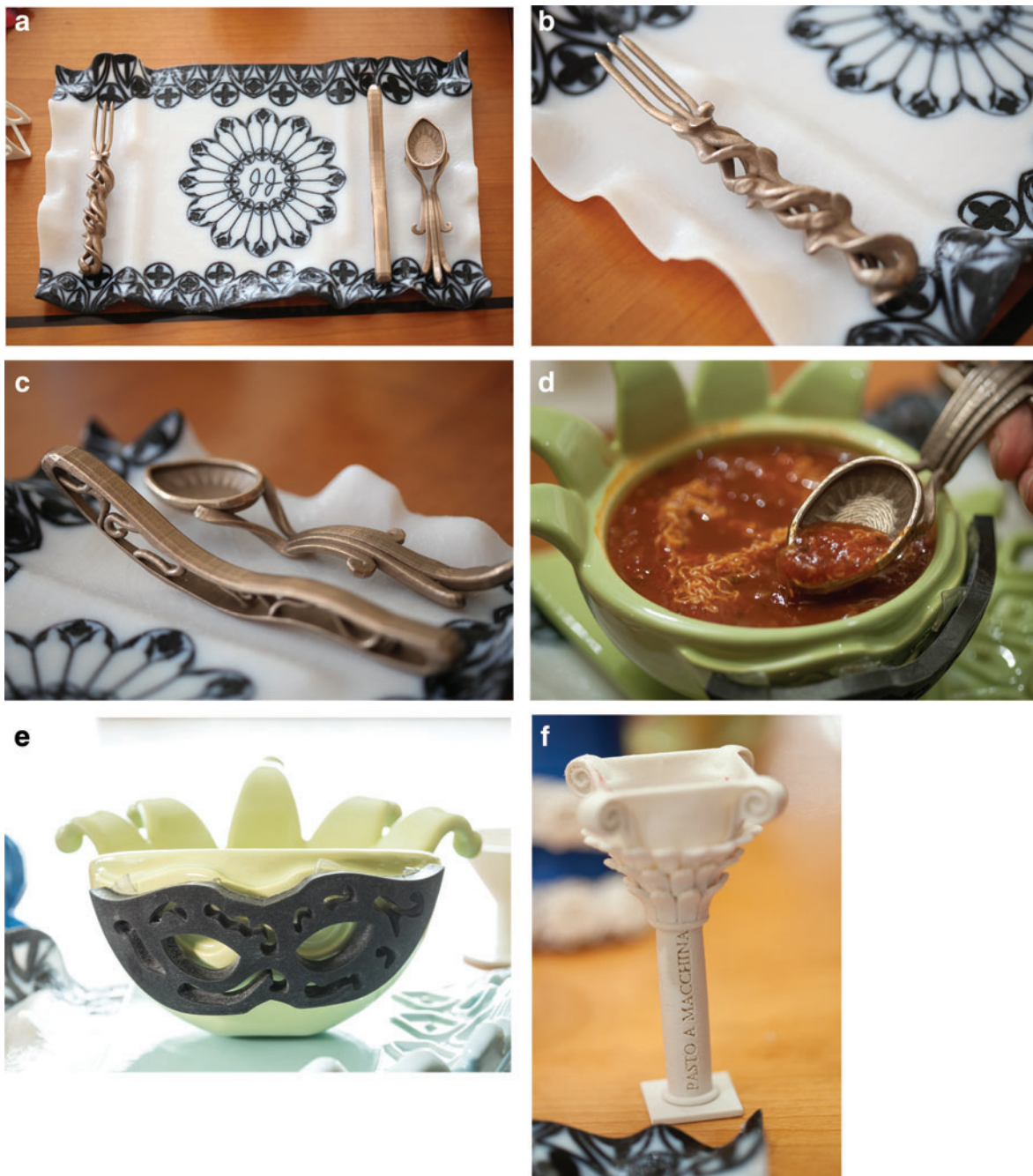
FIG. 1. Several items were produced using various 3D printing processes. The placemat (a) was produced on a Polyjet 3D printing system out of ultraviolet-cured resin. The system was then made food safe using a coating of silicone. The fork (b), spoon, and knife (c) were produced from stainless steel and coated to be food safe. The intricate designs would be difficult to produce using traditional processes. The unique design was made for a germophobic audience, having food contacting surfaces not resting on the table. The bowl (d) was produced using a ceramic printing process and designed to adjust its angle with the plate based on the soup content (e). This caused the bowls to tip away from the user and enforced proper etiquette. The wine glass (f) was produced using a fused deposition modeling system and coated with silicone to be watertight and food safe. Photographs credit of Tony Cenicola/The New York Times/Redux. Color images available online at www.liebertpub.com/3dp
