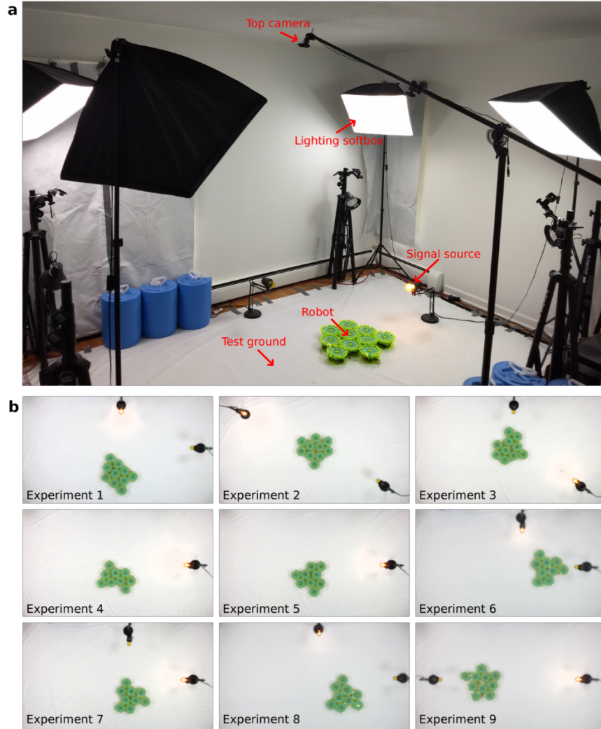
Figure S6: Locomotion Testing. (a) Experimental set-up for robot locomotion and (b) initial configurations of the nine locomotion experiments.
