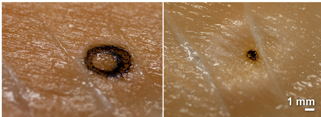
Fig. 5. Effect of laser beam flux on the salmon cooking results. Left panel: 1 mm thick salmon sample heated using a trochoidal cooking pattern with P = 2 \text{ W} , r = 2.5 \text{ mm} , T = 0.04 \text{ s} , \rho = 200 \text{ rev/mm} , and I = 2.71 \text{ MW/m}^2 . Right panel: 1 mm thick salmon sample heated using the same trochoidal cooking pattern except P = 5 \text{ W} , \rho = 80 \text{ rev/mm} , and I = 0.73 \text{ MW/m}^2 . Both patterns yield the same \omega ( 3.2 \text{ kJ/m} ) and \psi ( 16 \text{ MJ/m} ).
