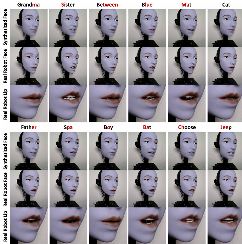
Fig. 4. Robot lip movements across different phonetic contexts. The figure presents synthesized predictions of the robot's lip shapes for various words alongside real-world robotic performance, illustrating how the learned model generalizes from simulation to physical execution.
